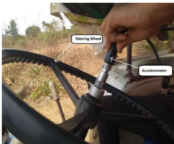
Fig.2. Accelerometer mounted on steering wheel
